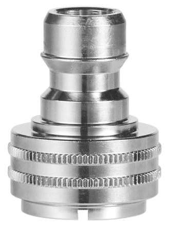
Fits water tap with  $\frac{1}{2}$ ",  $\frac{3}{4}$ " or M22 mm outside thread. When the bush is removed, the coupling fits a  $\frac{3}{4}$ " external thread. When the bush is turned upside down the coupling fits a M22 mm external thread.
